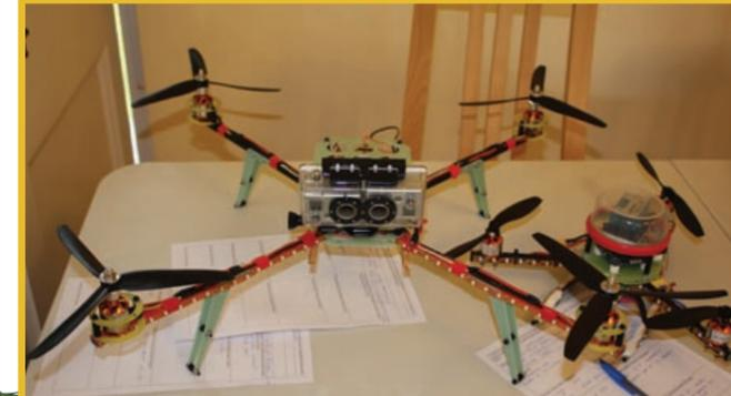
This quadcopter UAV features two GoPro cameras which when configured as a pair can be used for making 3D aerial recordings
